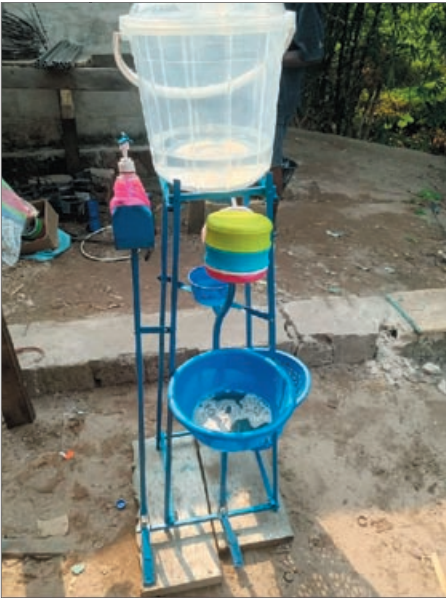
Mechanical pedal-operated hand-washing units which Joseph manufactures. R: An order from UNICEF shipped to the East of DRC.
