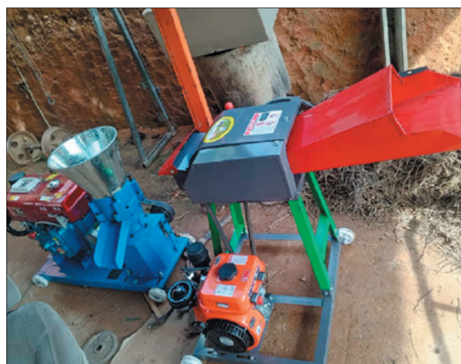
Machine for making pellets to feed animals and fish. The other is for grinding grass for livestock.
