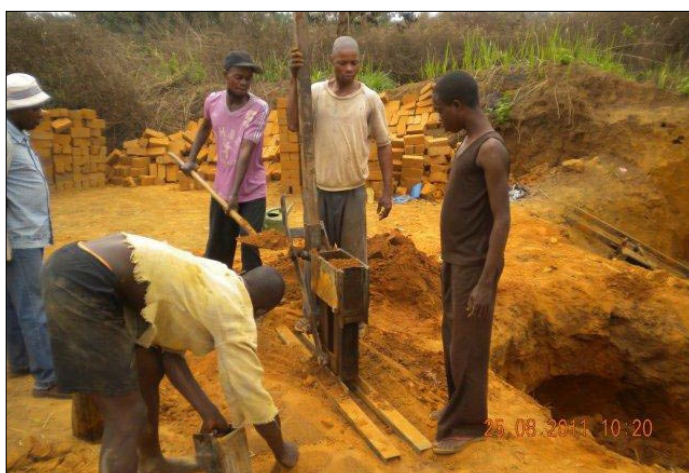
Machine for pressing bricks by hand: clay, a little oil & some elbow grease. After being burned they become very strong
