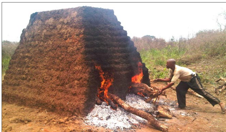
Simple brick oven: bricks stacked up high, covered with mud, fire inside
