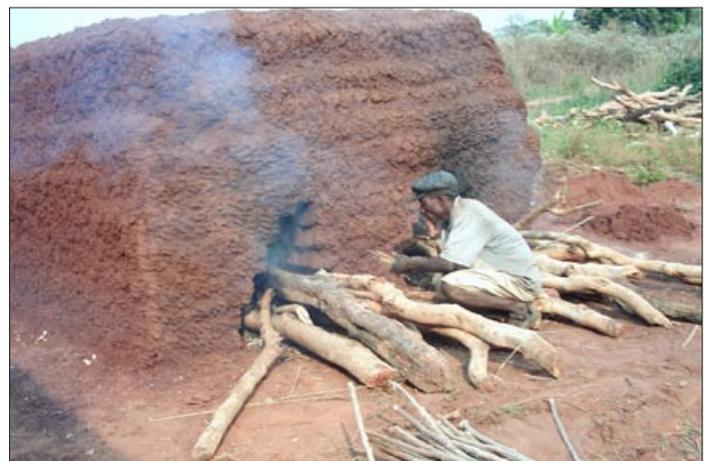
*Bricks being stacked up to an oven with 2 openings. After getting covered with much, fire is put inside and then sealed.*
